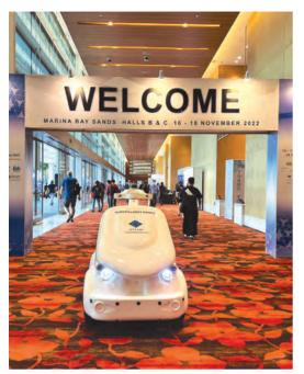
O-R3, OTSAW's autonomous security patrol robot at the exhibition. Photo credit: OTSAW
